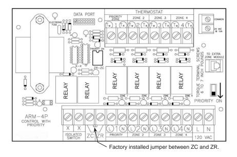
Each zone thermostat will signal the ARM control to operate its zone circulator and start the boiler through the XX isolated end switch.
