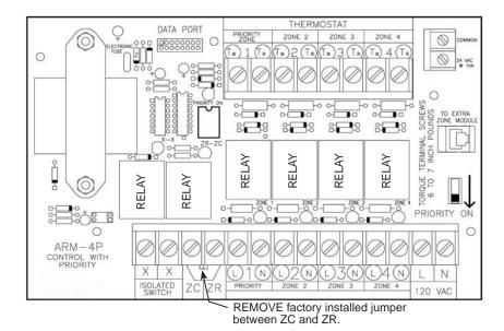
A tankless coil requires a boiler aquastat. Each zone thermostat will signal the ARM to start its zone circulator and send a call for heat to the boiler aquastat. If boiler temperature drops below the low limit setting, all circulating will cease until temperature of boiler water is increased.
